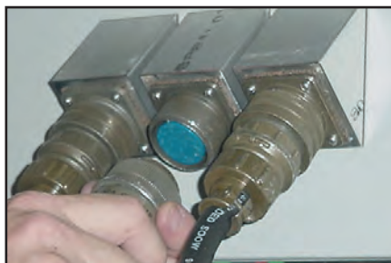
▲ Control cable connections
