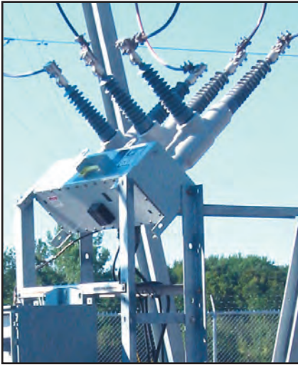
◀ Picture shows 45° angle mounting for applications requiring the same load and line side connector height.
