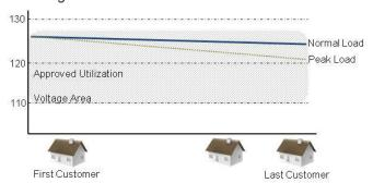
Lazer CVR software enables the automatic control of tapchangers and voltage regulators to optimize the voltage level. Using an interface to the AMI software and automated customer meters, the end of line voltage can be monitored in real time and the substation voltage regulated appropriately. This allows the power providers to save roughly 0.7% in power for every 1-volt decrease in voltage. Two examples of the software in action are:
