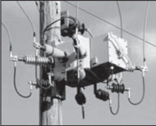
G&W's overhead Rotary Puffer (RP) switches are ideal for manual load break switching, standard speed (5 seconds per operation) automatic transfer or automated sectionalizing on systems rated through 27kV, 630A continuous, 32kA peak and 20kA asymmetrical short circuit. The switches are tested to applicable sections of ANSI and IEC standards.
