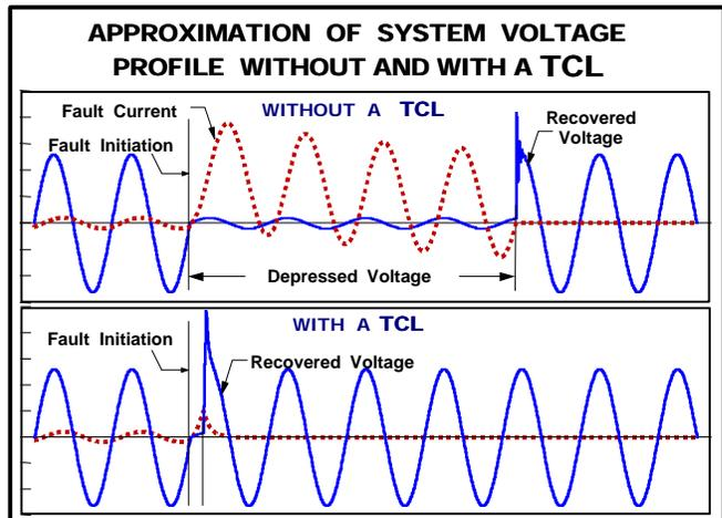
Figure 6: System Voltage During Fault
