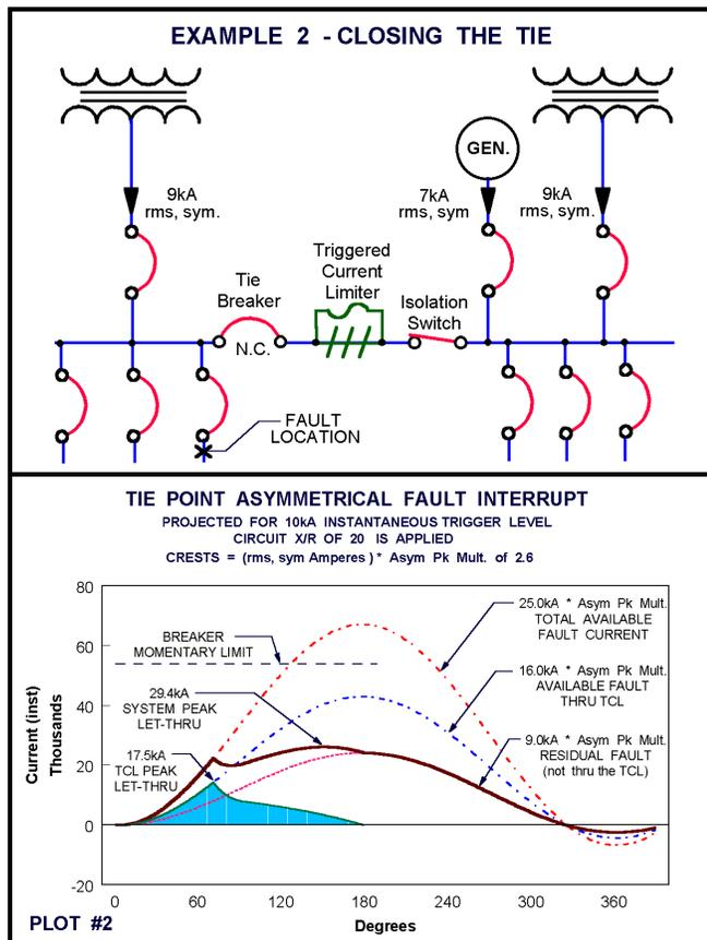
Figure 3: Example 2 and Plot 2 for Bus Tie Application
