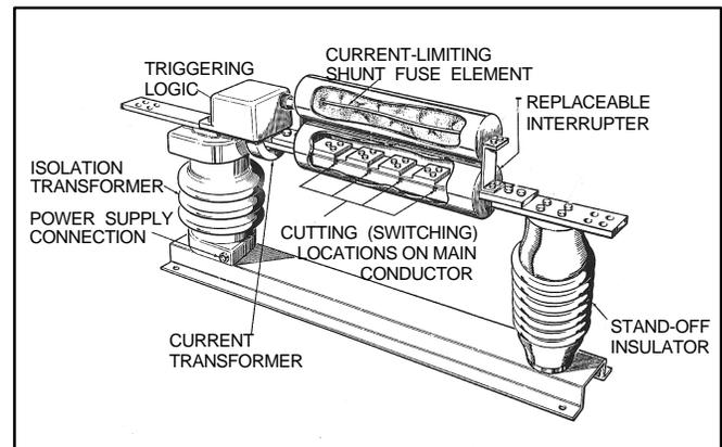
Figure 1. Layout of a Triggered Current Limiter
