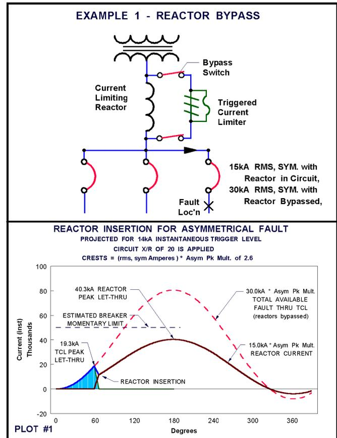
Figure 2: Example 1 and Plot 1 for Reactor Bypass
